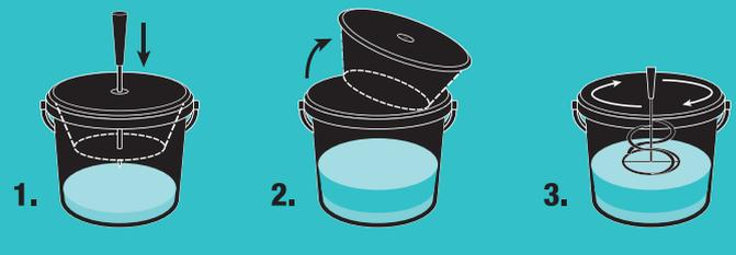
1. Pierce the centre of the lid on the top chamber and push through to pierce the centre of the base also. Allow the material (hardener) to fully drain from the top container into the base. This will normally take between 3 and 5 minutes.
