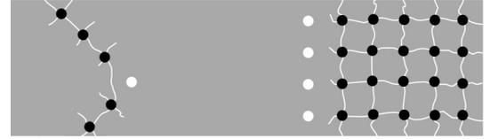
**Removing a layer of mother rock** begins with drilling a few smaller holes to remove the toe and obtain a regular, vertical free surface. Then more holes parallel to the new surface and reaching a few centimetres below the desired cut-off level are drilled. 2 consecutive rows are then filled up every 5 to 15 hours.
