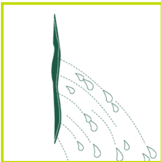
Leak through crack in wall or floor.
