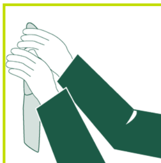
Apply the paste to the leak and hold firmly in position without movement until set.
